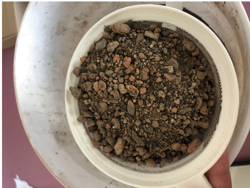
Figure 91. Load the soil sample in the strainer.
