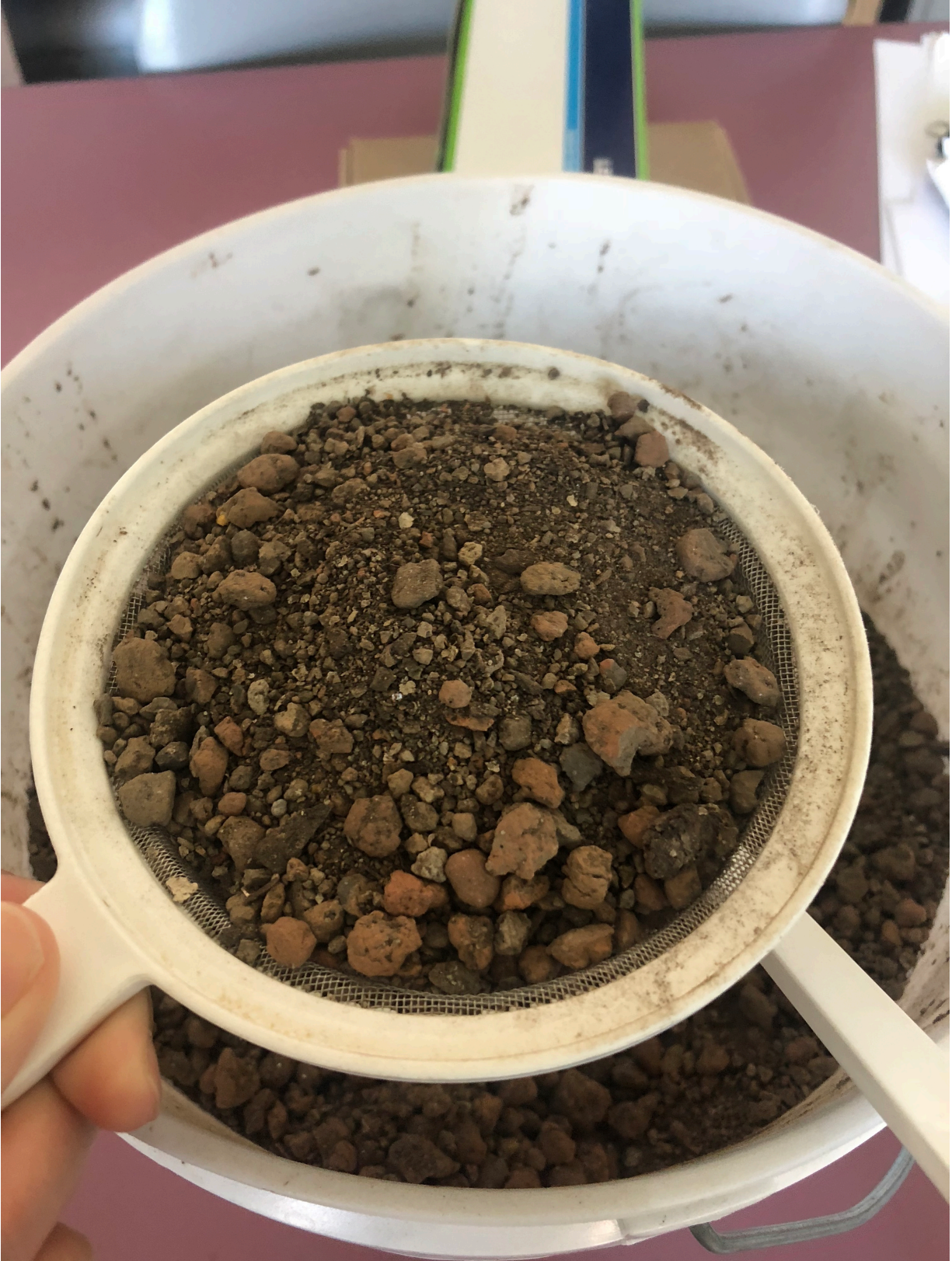
Figure 84. Load soil into the strainer.
