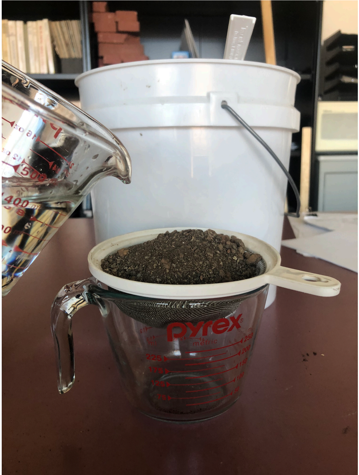
Figure 86. Place the strainer containing soil on the top of the measuring cup.
