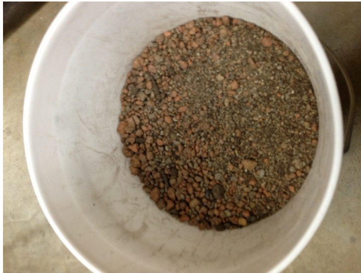
Figure 68. Dehydrated soil in bucket.
