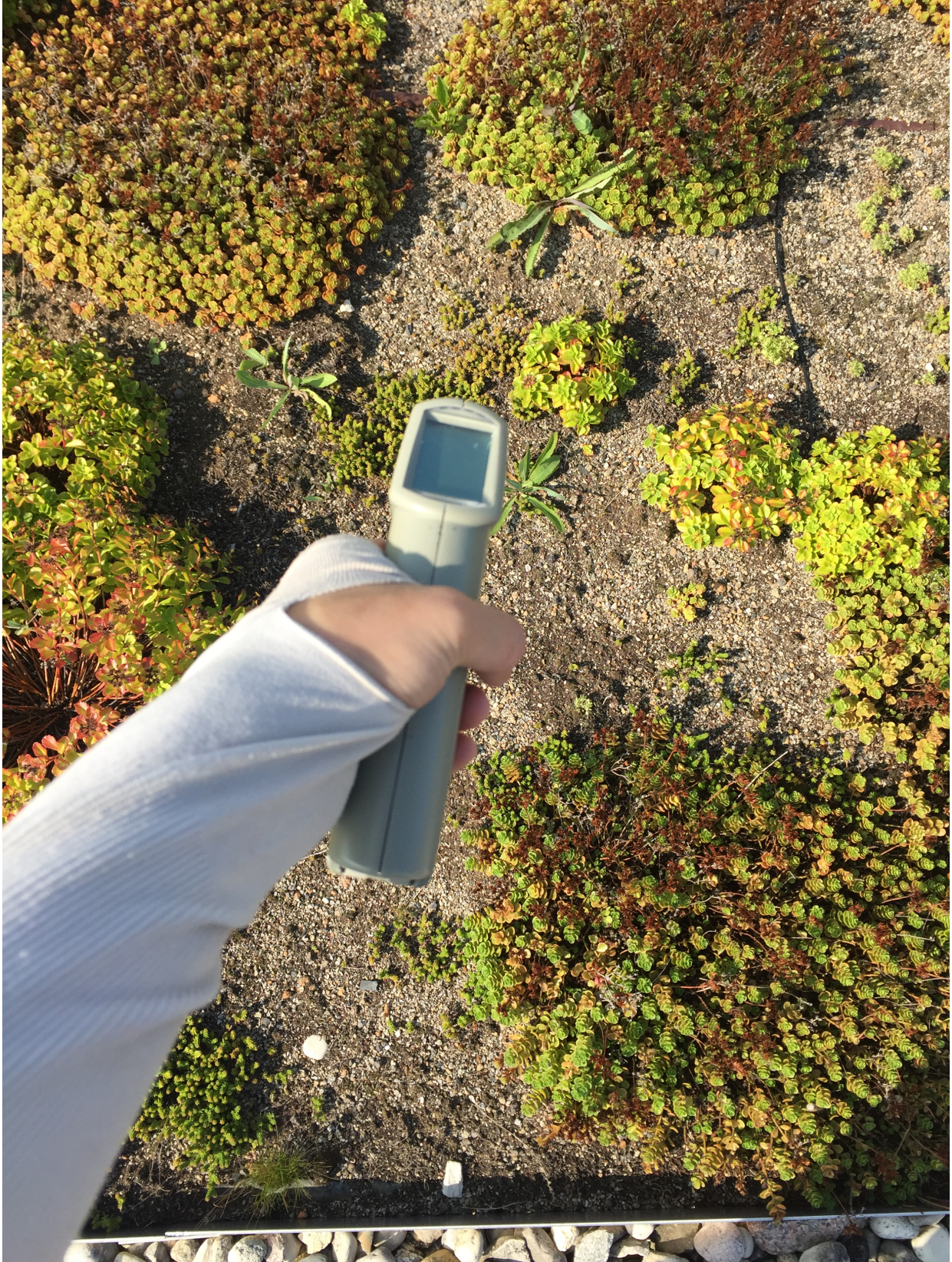
Figure 25. Measuring surface temperature with an infrared thermometer
